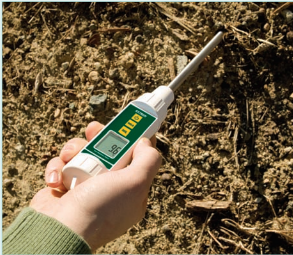
Check the moisture of soil content to insure healthy plant growth
