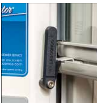
At left: The sprocket cam is revealed when the side panel and protective cover are removed. At right: The defeatable stop holds the sash fully open.
