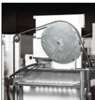
At left: The sprocket cam is revealed when the side panel and protective cover are removed. At right: The defeatable stop holds the sash fully open.
